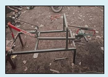
In this Pedal operated hacksaw machine which can be used for industrial applications and households needs in which no specific energy or power is needed. The power hacksaw machine which runs on human power, works on the principle of the conversion of rotational motion to oscillatory motion.
