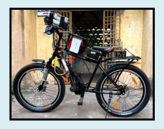
Bicycle is a two wheel vehicle, which is being powered by a rider and can be steered using a handle. It is one of the most eco-friendlier and an economical mode of transport word wide. One additional set of gears and chain was installed to increase the speed and reduce the effort of peddling as compared to normal cycle. It can travel more distance than normal cycle at same speed of peddling.
