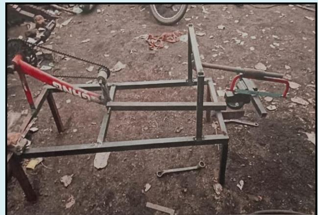
In this Pedal operated hacksaw machine which can be used for industrial applications and households needs in which no specific energy or power is needed. The power hacksaw machine which runs on human power, works on the principle of the conversion of rotational motion to oscillatory motion.
